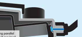
Ensure the silicone is sitting parallel on the hole below it. Hold at eye level to check the position is correct
